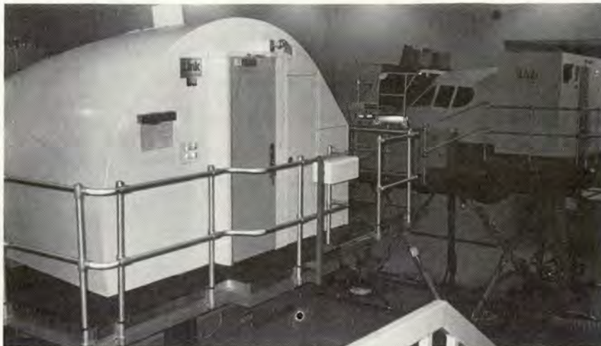
Towering on hydraulic struts, the weapon system trainers used by the 93d Bombardment Wing are described as the most complicated and advanced simulators ever produced. They allow very realistic simulation of past mishaps for extremely effective training.
